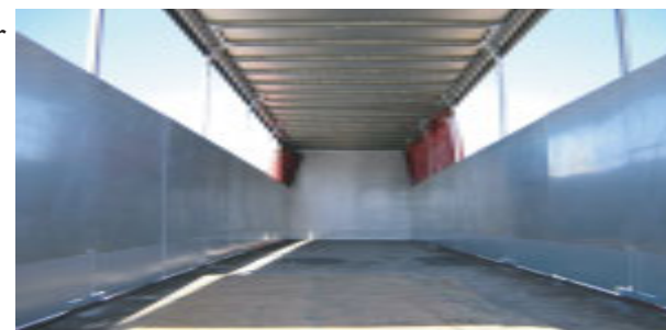
Aluminum Slide-A-Gates make an internal wall.
