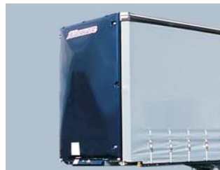
New Full Length Nose Cone – improved aerodynamics and fuel usage
